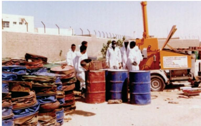
*Drum-crushing in progress, using a commercial drum-crushing unit*
