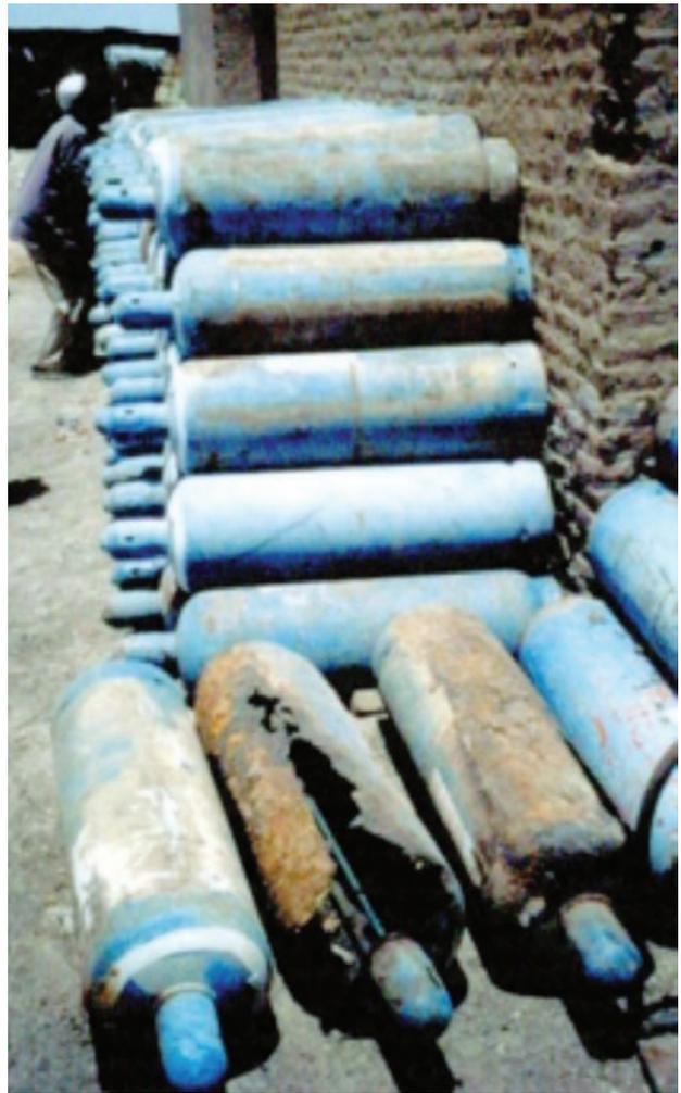
*Badly corroded pressure containers*
